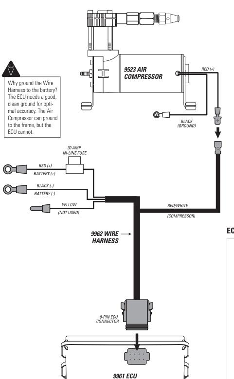
Route the Wire Harness in the most protected manner possible, and securely make all connections as shown.
