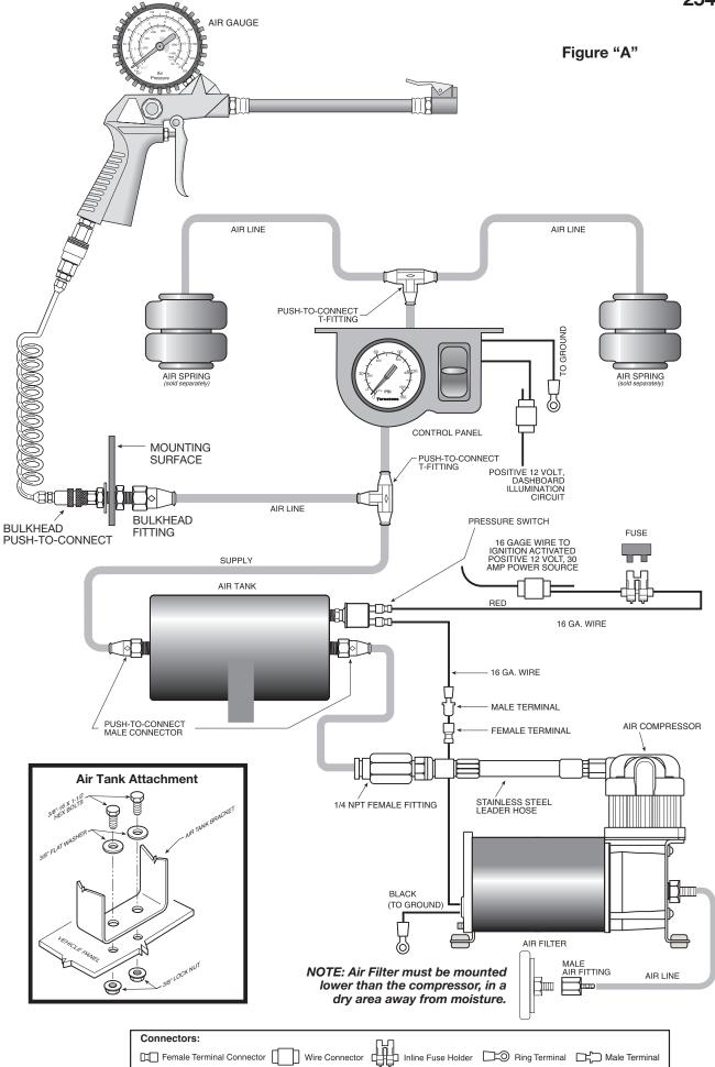
should be rigid to support the compressor, such as under the hood on a fender well or in a vented storage compartment. The compressor is oil-less and can be mounted in any orientation necessary for installation.
