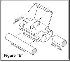
wire. Install the female spade connector over the remaining spade on the pressure switch. Connect the opposite end of the pressure switch wire to the 12 Volt power wire using a wire connector. Slide the wire connector over the existing wire and insert the un-stripped wire from the pressure switch into the wire connector. Close the wire connector over both wires with pliers **see Figure "E"**.
